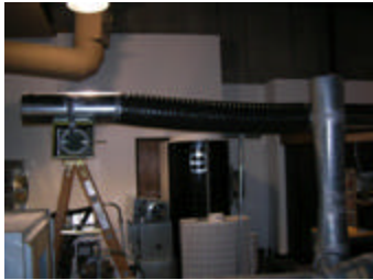
Fig. 1 Straight Duct (base line test)
